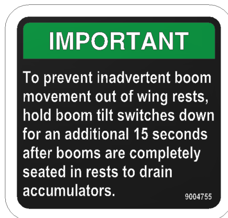
Part No. 9004755 - IMPORTANT (Accumulator Drain)
